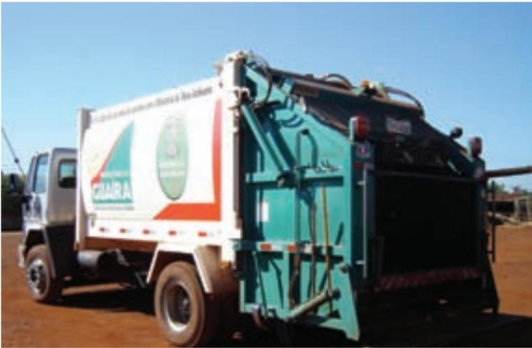
**FIGURA 6** - VEÍCULO PARA COLETA REGULAR, TIPO COMPACTADOR.
